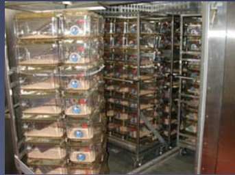
Three-shelf Rutgers carts Note top bar to support a cart cover
